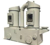
Packed bed scrubbers are effective for removing gases, such as acid gases (e.g., sulphur dioxide) and ammonia, as well as for controlling odours and certain volatile organic compounds (VOCs). They are commonly used when gas-liquid contact and mass transfer are required for effective pollutant removal.
