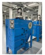
shock of air through the bag that shatters and discharges the dust cake for disposal. The rapid pulse of air allows for continuous operation with the fan running, and because of it the system is not generally compartmentalized. Pulse jet models are the most common type of industrial dust collectors, due to their ability to be easily customized, capability to handle a wide range of temperatures and pressures, and their
