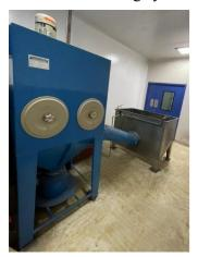
The dust collector is of Pulse Jet Type whereby the cleaning is done automatically by compressed air through a timer and solenoid valve. The filters shall be Cartridge type made out of spun bound Polyester with anti-adhesive finish.
