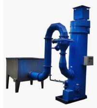
The scrubbed liquor is collected in the bottom recirculation tank which has to be drained periodically.
